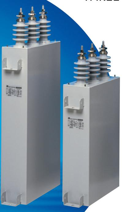
High voltage power capacitors are designed and manufactured by using latest technology and high quality materials. They have all-film dielectric and are impregnated with dielectric liquid which is biodegradable in environment. Each capacitor element has a separate internal fuse. In addition, each capacitor is provided with an internal discharge resistor.
